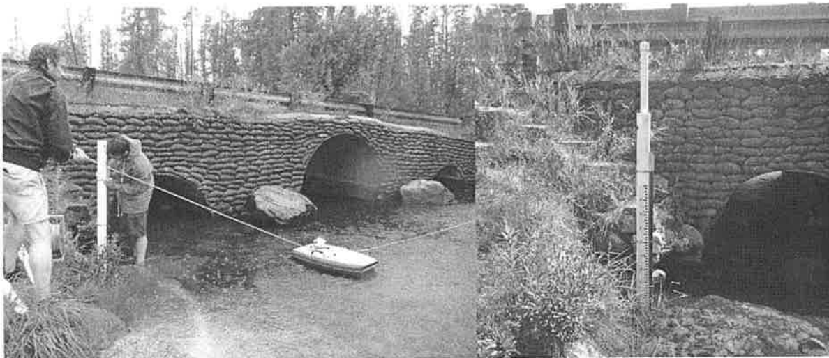
Figure 4.1.1. Installation of a stream gauge and discharge measurement on the Cut River at West Lansing Road (Site HL-CR-2).
