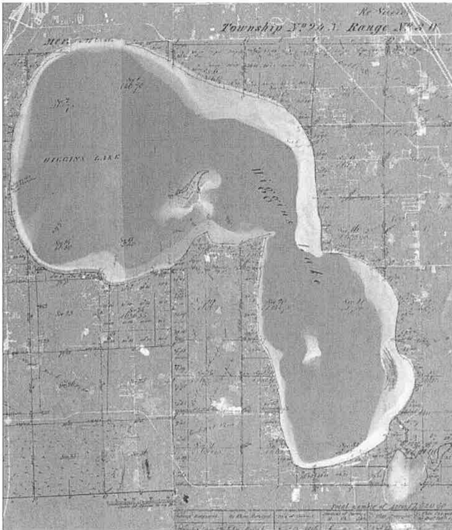
Figure 1.8.1. The original Higgins Lake survey from the Michigan public land survey plat maps from the mid 1800's. The plat map was georectified using aerial imagery underlay, provided by the USDA, taken on August 31 and September 1, 2012.
